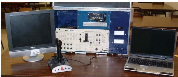
Surface Control System with Video Mixer, Video Selector, Fiber Mux, Power Supplies and PC
