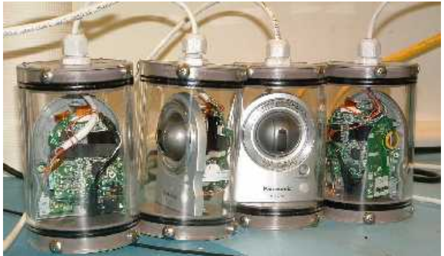
Figure 18 All Four Ethernet Cameras in Housings
