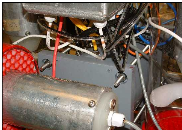
Figure 3 Side of ROV with Pneumatics Enclosure
